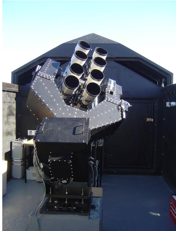
Figure 3.1: Photo showing the SuperWASP instrument, its robotic mount supports eight 11.1 cm refractive telescopes. We also see the roof which automatically opens and closes. Photo courtesy [www.superwasp.org](http://www.superwasp.org).
