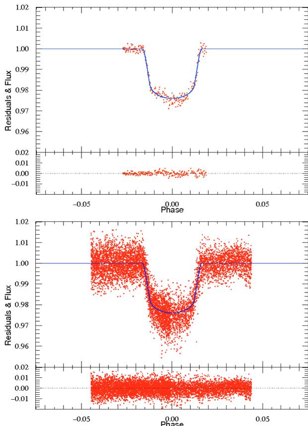
**Fig. 2.** FTS  $i'$ -band (top) and LT/RISE  $V+R$  (bottom) transit photometry for WASP-6 and residuals after subtraction of the best-fit transit curve (superimposed in blue).
