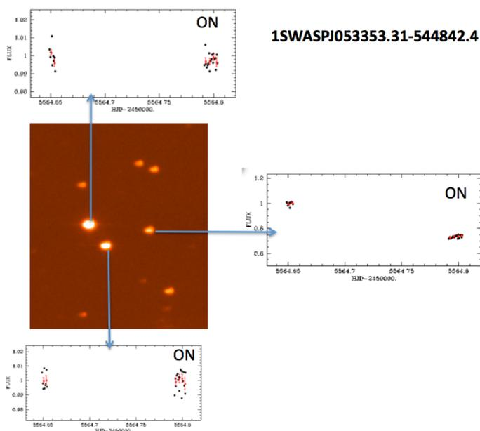
Figure 3.10: This WASP candidate had two bright star within the smallest aperture and seven altogether within the largest aperture. Michaël Gillon used the 70 cm TRAPPIST robotic telescope to observe in transit (*On*) and out of transit (*Off*) and determine which of the star was being transited. In this case a faint nearby star shows a 20 % depth eclipse. Not a planet. Plot & analysis by Michaël Gillon.
