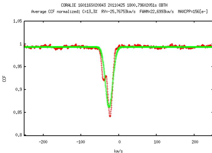
Figure 3.13: CCF and Gaussian fit as outputed from the DRS. Here the case of a blended double line binary (SB2). A second peak is clearly resolved. The deeper CCF (the primary) is seen moving from another epoch by several  $\text{km s}^{-1}$ . This system is probably an fairly short period binary ( 20 day period). The transit WASP detected is most probably on the primary.
